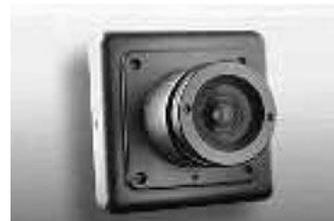
Figure 2: The Sony CCD digital camera
