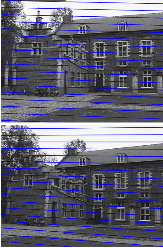
Figure 5: Two frames from the 'Castle' sequence, with epipolar lines overlaid
