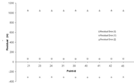
Figure 2. The error plot in X,Y,Z in no-GCP scenario
