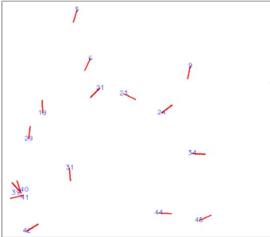
Figure 7. Error vectors of check points measured on Orthoimage (magnified 400 times).
