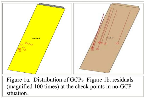
Figure 1a. Distribution of GCPs Figure 1b. residuals (magnified 100 times) at the check points in no-GCP situation.
