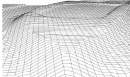
Figure 2: Filtered DTM without extracted break lines
