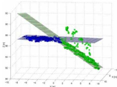
Figure 4: Example of adjusted plane pair using robust least-squares (vegetation is filtered, cf. Briese, 2004b)
