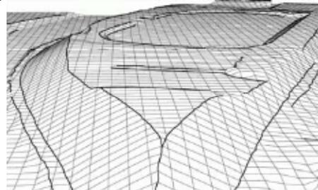
Figure 3: Filtered DTM including extracted break lines
