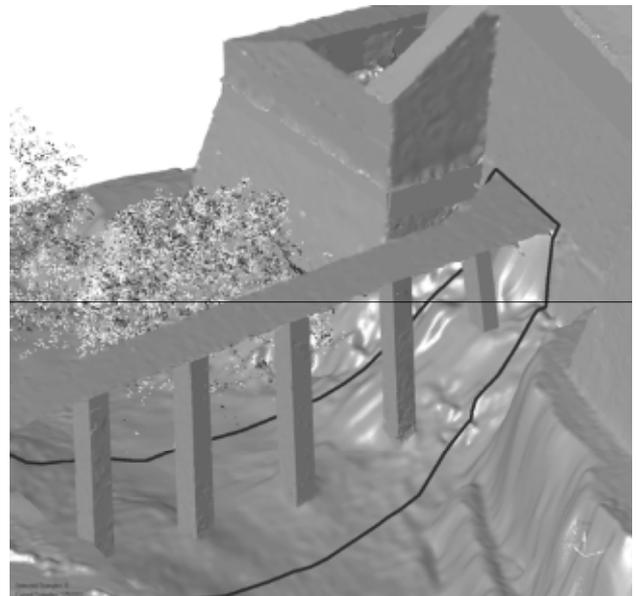
Figure 11: Test scene including a 3D bridge enclave. Also visible the enclave boundary (black) and as vegetation classified point data (bright dots)
