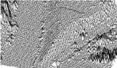
Figure 1: Triangulation of the unfiltered point data
