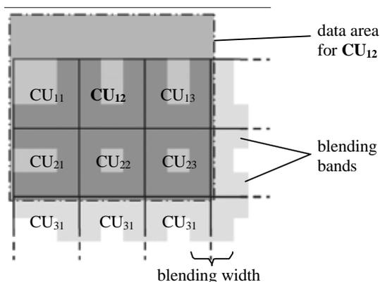
Figure 5: Computing units with blending bands
