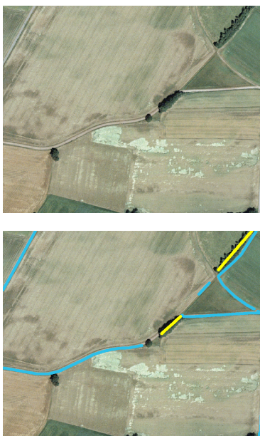
Figure 4: Object extraction. Upper: image, lower: extracted roads (blue) and extracted rows of trees (yellow).
