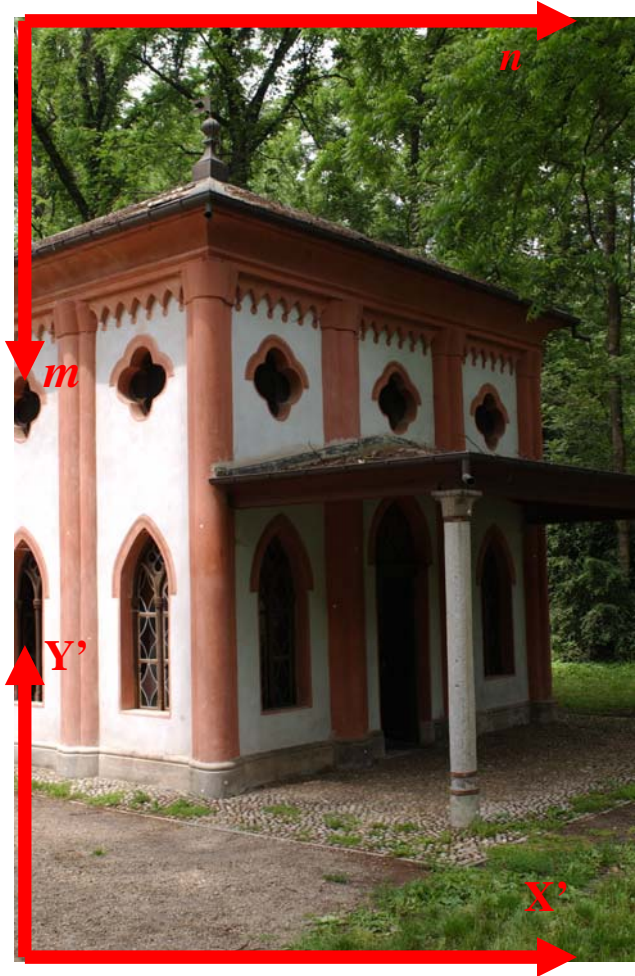
Figure 4. Digital image internal reference system (above) and dummy system used for the georeferentiation (below)
