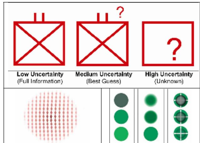
Figure 2. Selected symbols and cartographic methods for visualising levels of uncertainty: Tactical icons (top; St. John et al., 2000), blurred icons (bottom, left; Kim and Kesavadas, 2004) and point symbol sets (bottom, right; MacEachren et al., 2005)
