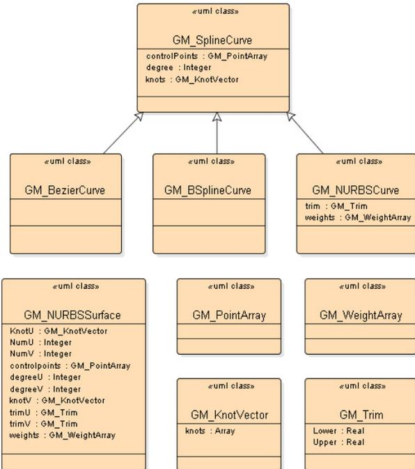
Figure 2: UML schema of four implemented data types (GM\_BSplineSurface and GM\_BézierSurface are not shown)
