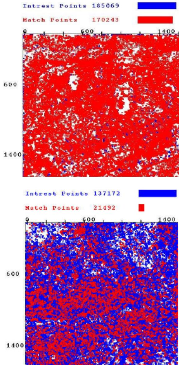
**Figure 2:** Comparison of the image match points as obtained from stereo pair I and pair II. Note the poor image matching in stereo pair II.
