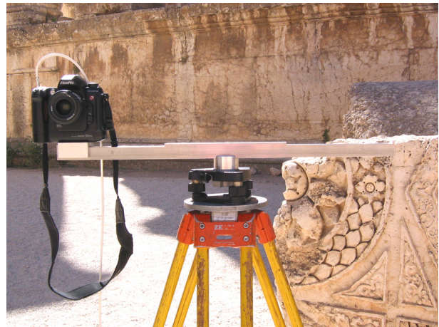
Figure 2. Simple camera bar for stereoscopic exposures with defined base distances of 30 cm and 60 cm
