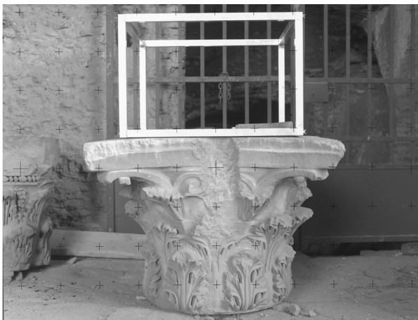
Figure 4. Reference frame for stereo model orientation, (Corinthian capital, object height 80 cm, Rollei 6006 metric, c_k 80 mm, scan 2500 dpi)
