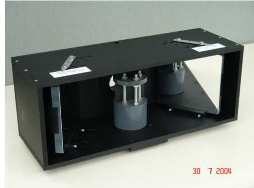
Fig. 2: Prototype of a mirror-based stereo camera
