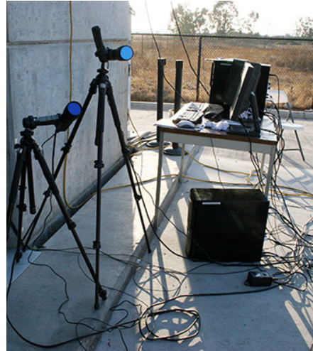
Figure 3. ShapeMonitor system with 2 of the 4 cameras with filters on lenses
