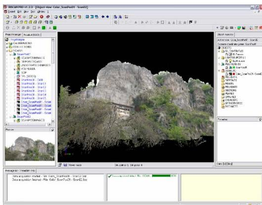
Figure 5. Acquisition Software - RiscanPro - Riegl – scan position 01.
