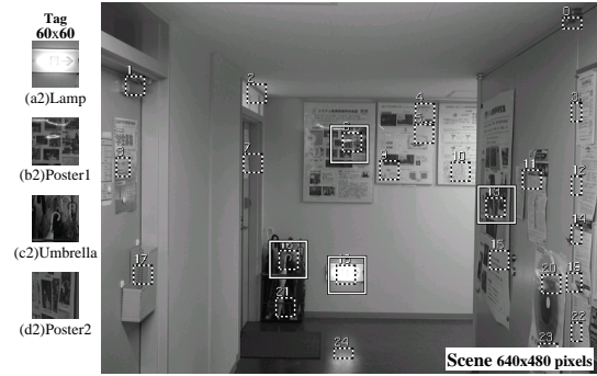
Figure 14: (a2) is a reference image which picks up an isolated object and used to estimate a scaling factor. (b2), (c2), (d2) are searched using the scaling factor in a scene image.
