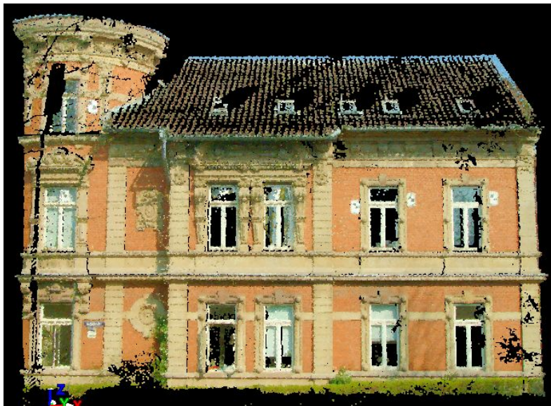
The textured façade free from the different types of the occlusions (textured using the three photos)
