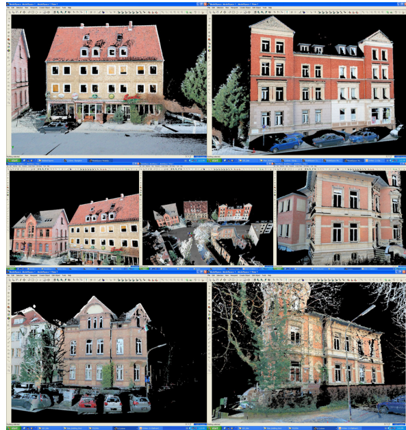
Figure 10: Some snapshots for the crossing true colored point cloud displayed in the cyclone software
