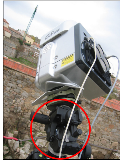
Figure 1. Trimble GS200 laser scanner ( www.trimble.com ) and micrometric head (red circle).
