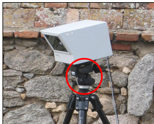
Figure 2. Ilris 3D (Optech) laser scanner ( www.optech.ca ) and micrometric head (red circle).
