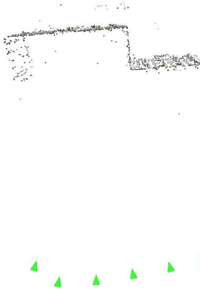
Figure 2. 3D points (red) and cameras (green pyramids, the tip symbolizing the projection center and the base giving the direction of the camera) derived from the images given in Figure 1
