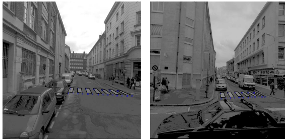
(a) 7 bands out of 7 are detected and correctly reconstructed (b) 6 bands out of 6 are detected. 1 band is not correctly reconstructed due to non-flat band
