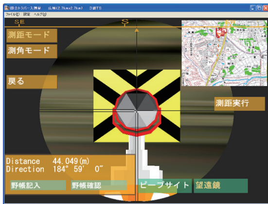
Figure 8. Collimation by telescope
