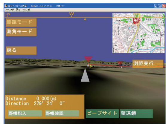
Figure 7. Collimation by peep sight
