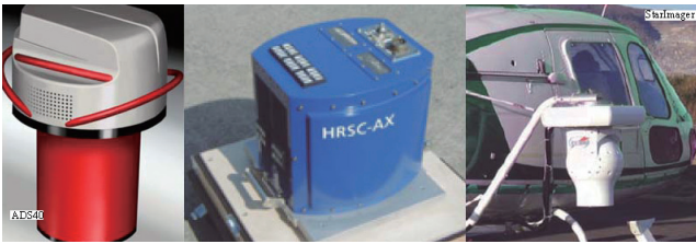
Figure.4: Airborne Linear Cameras: ADS40-HRSC-AX-StarImager
