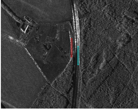
Figure 5. SAR image with coloured rectangles, each marking an azimuth line used for building a FM-azimuth slice
