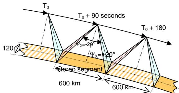
Figure 1. SPOT-5/HRS along-track image acquisition
