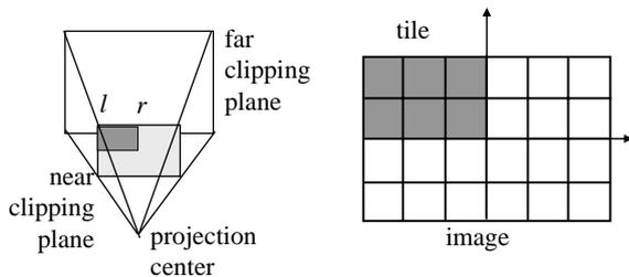
Figure 6: Projection of tiles and the corresponding OpenGL parameters, which are computed during the real time loop.
