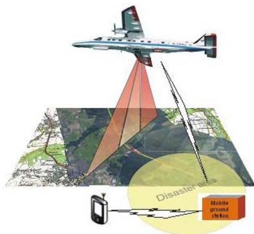
Figure 1: One application scenario for a wide area high resolution airborne camera system.
