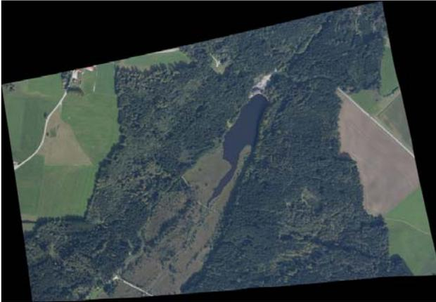
Figure 12: Orthoimage computed with the same original image and with the equal DSM. The entire image is projected according to (Mueller et. al. 2004).
