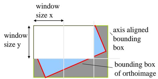
Figure 7: Scanning the high resolution image, here six rendering steps are required in the inner real time loop.
