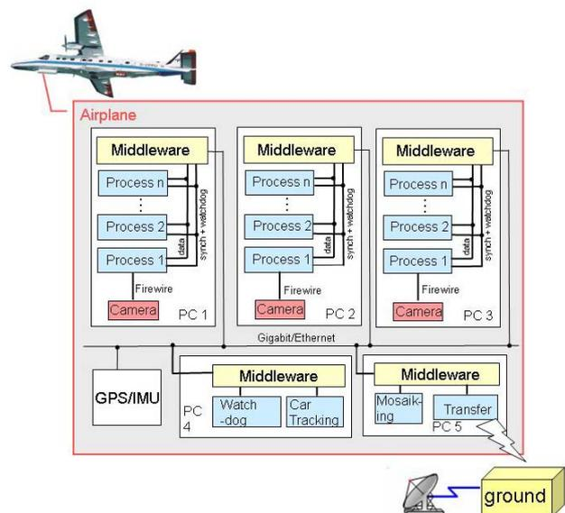
Figure 3: Architecture of our distributed real time on-board system.
