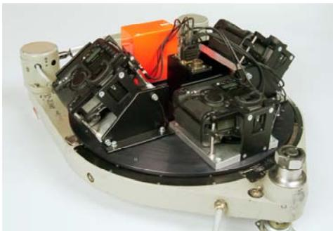
Figure 2: DLR 3K-camera system consisting of three Canon EOS 1Ds Mark II, integrated in a ZEISS aerial camera mount.
