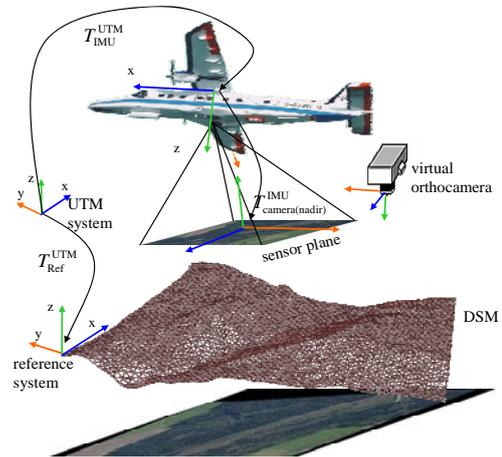
Figure 5: Arrangement in 3d. All transformations are depicted. The RPY angles are obtained by the GPS/IMU.
