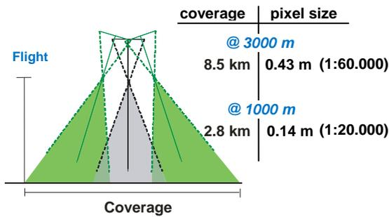
Figure 4: Illustration of the image acquisition geometry. The tilt angle of the sideward looking cameras is approx. 35°.
