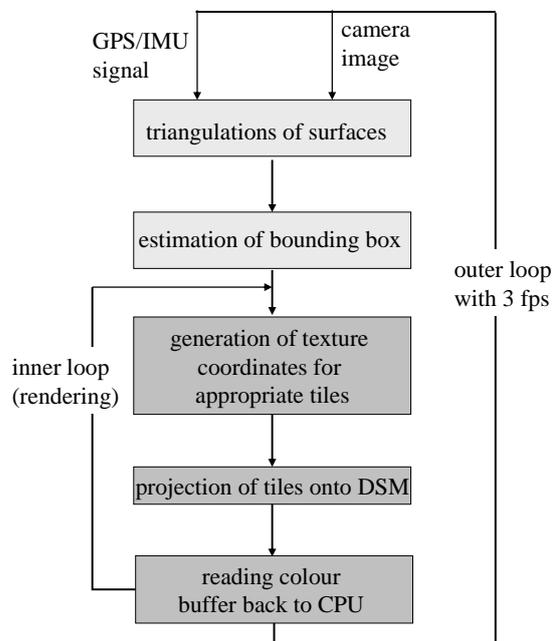
Figure 8: Processing steps to be computed within the real time loop. Each projected image is assembled to the final ortho-image.
