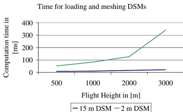
Figure 9: Computation times for loading and triangle DSMs on-the-fly in according to flight height for our DLR 3K-camera system.
