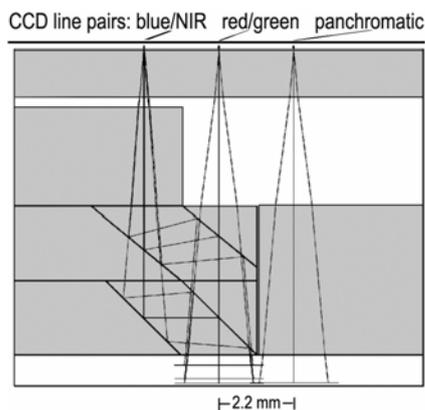
Figure 1. The Tetrachroid, glass shown in grey
