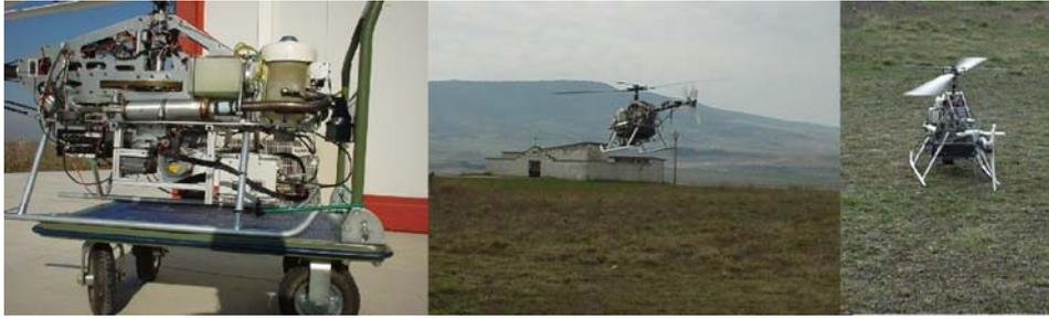
Figure 1: An AIN's UA with the IG's PRS sensor and navigation-orientation payloads: GPS L1/L2 receiver, LN200 IMU, Hasselblad Biogon SWCE 903 and the PRS navigation-orientation Control Unit. (Photographs courtesy of AIN.)
