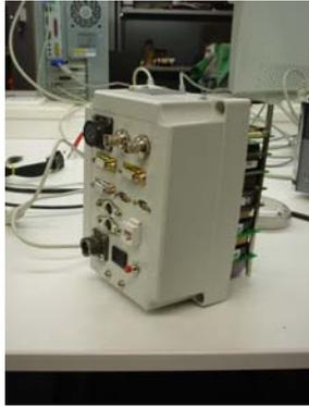
Figure 2: IG's PRS navigation-orientation Control Unit based on the PC104 architecture ( $\approx 13 \times 20 \times 18$  cm<sup>3</sup>,  $\approx 2$  kg).
