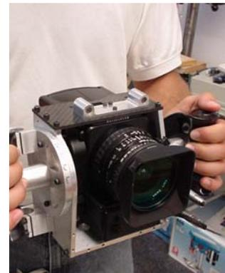
Figure 3: EPFL's Hasselblad Biogon SWCE 903 ( $\approx 17 \times 21 \times 17$  cm<sup>3</sup>,  $\approx 5$  kg).
