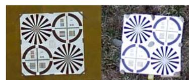
Figure 4: Siemens star target from a distance of 20 m [preliminary results].
