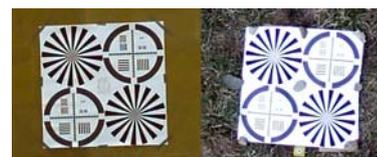
Figure 4: Siemens star target from a distance of 20 m [preliminary results].
