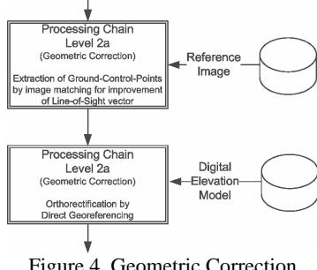
Figure 4. Geometric Correction
