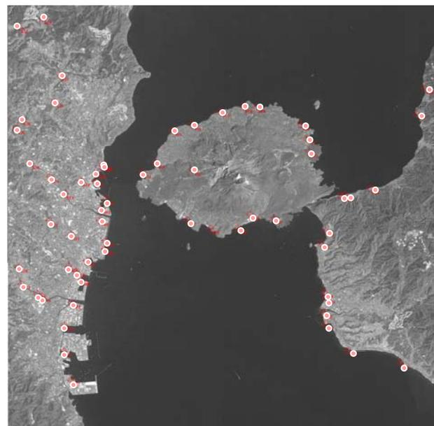
Figure 2. GCP distribution over the Cartosat-1 Aft image of the Sakurajima test site
