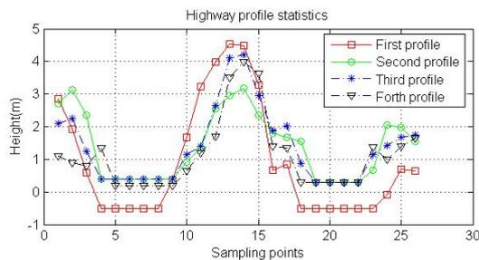
Figure 3. Highway's profile sampled on different sections (the sampling points with a certain distance)
