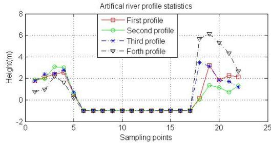
Figure 2. Artificial river's profile sampled on different sections (the sampling points with a certain distance)
