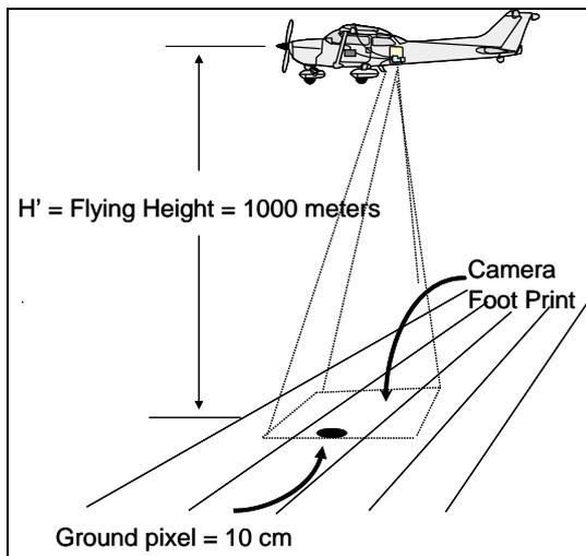
Figure 1. calculation of GSD for the Intergraph DMC
