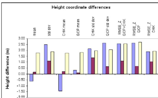
Figure 9. Statistics regarding the Height coordinate differences ( $Z_{2003}-Z_{2001}$ ) measured on the two blocks oriented according to the three proposed methods.
