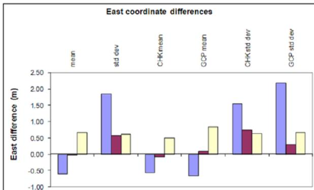
Figure 8. Statistics regarding the East coordinate differences ( $E_{2003}-E_{2001}$ ) measured on the two blocks oriented according to the three proposed methods.
