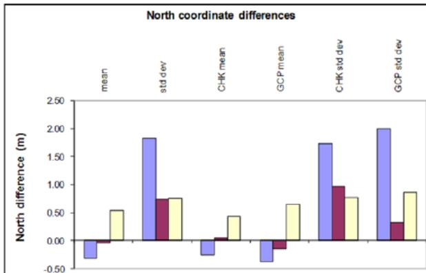
Figure 7. Statistics (relative accuracy) regarding the North coordinate differences ( $N_{2003}-N_{2001}$ ) measured on the two blocks oriented according to the three proposed methods.
