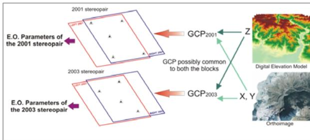
Figure 2. The Single Block Bundle Adjustment concept.
