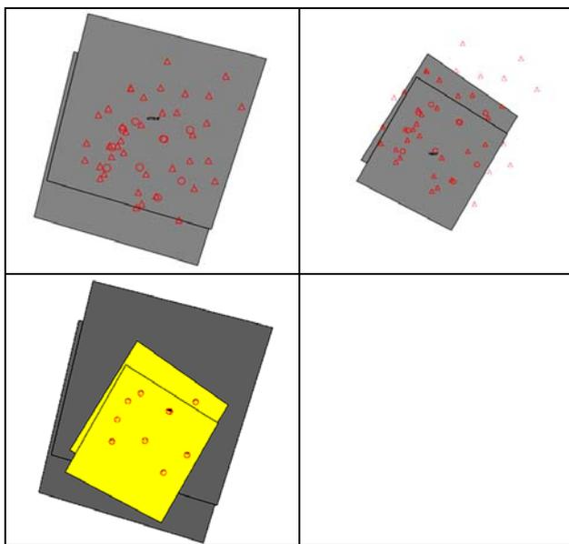
Figure 5. Upper Left: 2001 oriented model footprint; Upper right: 2003 oriented model footprint; Lower Left: 2001 and 2003 blocks, with the only CHKs overlaid. Triangles = GCPs; Circles = CHKs.
