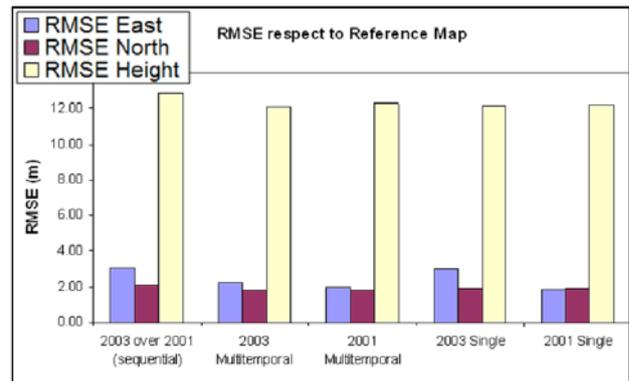
Figure 10. RMSEs globally calculated for the joined set of points CHKs + GCPs. Results refer about the difference between the coordinates of the points as estimated by each single oriented model and the reference ones (as measured on the reference map data). Estimations are labelled (X-axis) according to the adopted adjusting method used.
