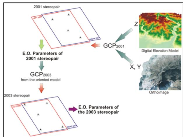
Figure 3. The Single Block Sequential Bundle Adjustment concept.
