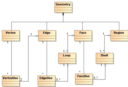
Figure 1. 3D spatial data model based on the principle of cell complex
