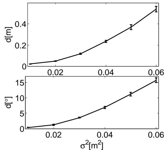
Figure 9: Distances of the first and last frame of the synthetic test sequence plotted against the variance of the image noise. *Top*: Distance between the projection centers of the two cameras. *Bottom*: Angular distance between the viewing directions of the two cameras.
