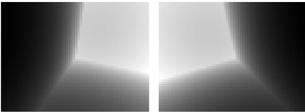
Figure 7: First and last depth image of the synthetic test sequence. It shows a rectangular corner at a distance of  $3m$  in front of the camera, which is moved  $4m$  to the right keeping the corner centered.
