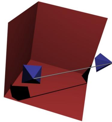
Figure 8: The 3D setup of the synthetic corner test sequence. The corner is  $3m$  in front of the camera. Then the camera was moved to the right  $4m$  keeping the corner centered and then back again, so that the final pose of the camera should coincide with the first.
