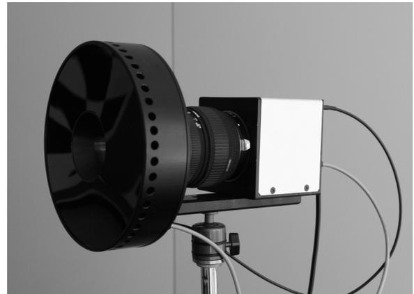
Figure 1: The Zess MultiCam PMD camera. Modulated infrared light is emitted from the front ring and the depth is measured using the Photonic Mixer Device behind it. The resolution is  $64 \times 48$  pixels and the opening angle is approximately  $18^\circ \times 14^\circ$ .
