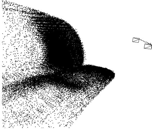
Figure 6: Final 3D point cloud after 100 images now comprising of 307200 points. The camera trajectory is shown as well.
