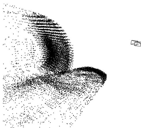
Figure 5: Intermediate 3D point cloud and camera trajectory. The point cloud has become more dense due to the movement of the PMD camera.
