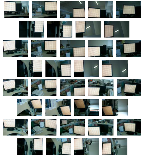
Figure. 3. Calibration Images shot at four positions, each position includes 9 photos
