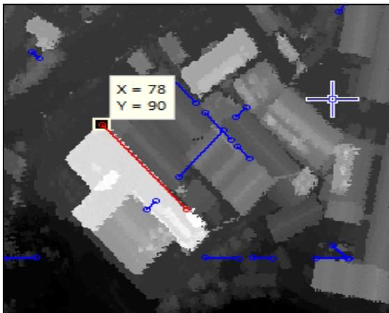
Figure 2. Manual selection of extracted 3D line features
