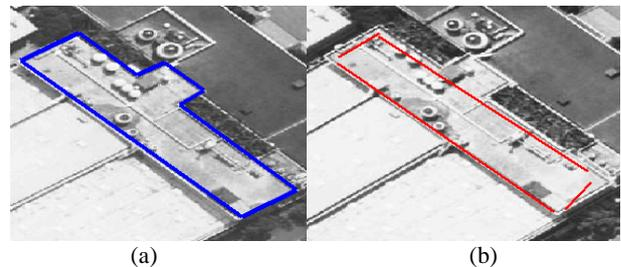
Figure 16. Updating the building roof model
