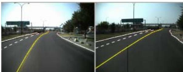
Figure 14: Example of miss detection to worn-out lane line
