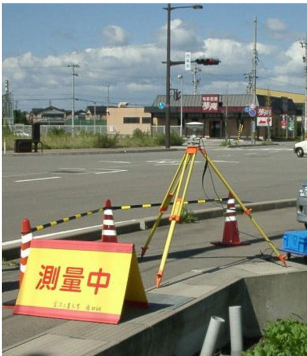
Figure 2. GPS measuring at the field point
