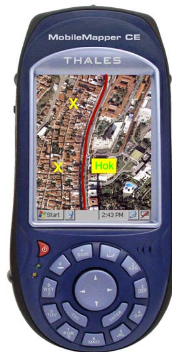
Figure 8. Handheld based Mobile GIS with editing and navigation function can assist in Crisis management for updating the GIS Database and navigate. [Example from GGS-Speyer, 2008]
