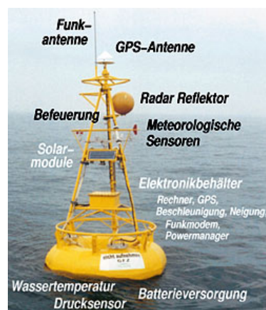
Figure 8. Tsunami Sensors installed close to tectonic fault zones for detecting Tsunami waves when they start, [http://www.forschung.bmbf.de/de/4879.php accessed on 18.04.08)
