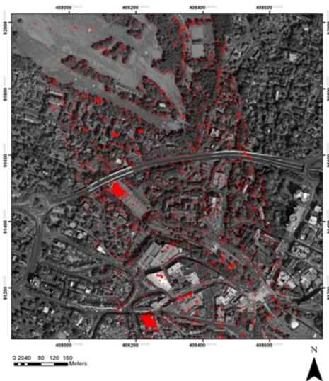
Figure 11 A point to node comparison highlighting change between 2005 and 2006 Bournemouth datasets.
