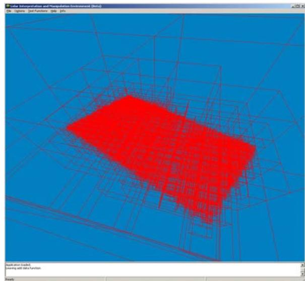
Figure 1 An octree generated from data used in the study
