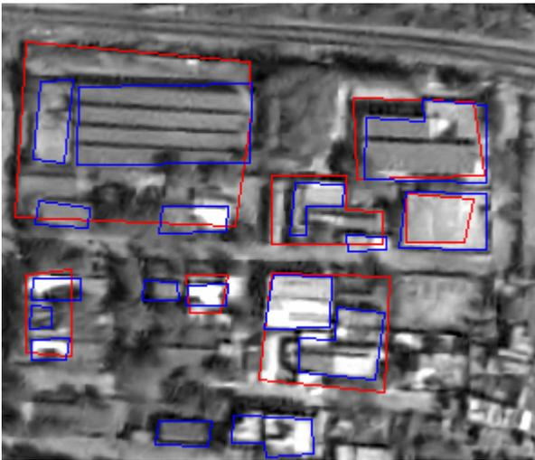
Figure-2(b) Overlay of features extracted in 2D mode (Red: Cartosat-1 & Blue: Cartosat-2) over Cartosat-2 ortho-image
