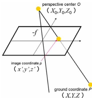
Figure 2: Simple photogrammetric model.
