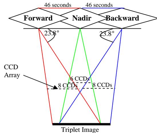
Figure 1: Scan geometry and triplet image of PRISM sensor
