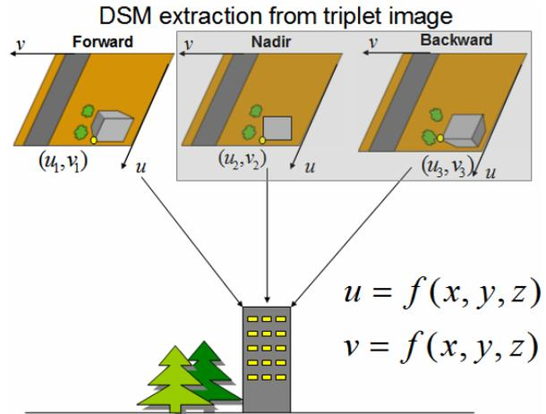
Figure 3: DSM extraction from PRISM data.
