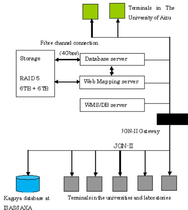
Figure 1. The system design of our WebGIS-based collaboration environment.
