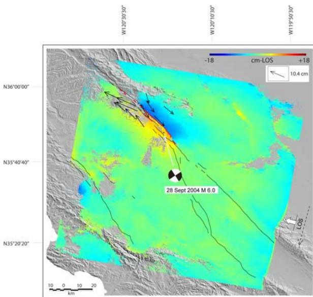
Figure 4. Unwrapped coseismic ERS-2 interferogram. Surface deformation in the LOS direction is consistent with a dextral strike-slip mechanism. The inferred surface rupture
