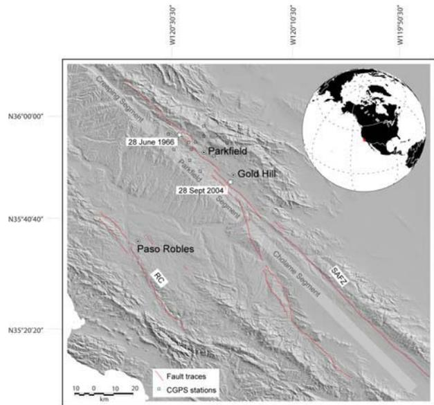
Figure 1. Map of the Parkfield region studied in this paper. It shows the location of major faults and continuous GPS sites. SAFZ stands for San Andreas Fault Zone and RC for Rinconada Fault. We plot the epicenters of the 1966 and 2004 earthquakes as white stars. Topography is from the Shuttle Radar Topography Mission (SRTM) (Farr et al., 2004) digital elevation model.
