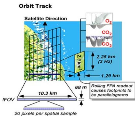
Figure 1 OCO ground track and field of view. The IFOV contains eight footprints in this diagram. Footprints are not rectangular because of the timing of the focal plane read out.
