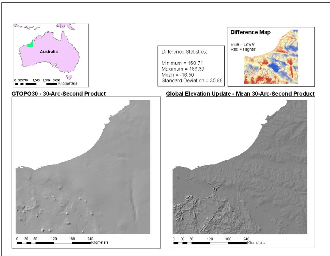
Figure 8. Comparison of the New Mean and Existing GTOPO30 30-Arc-Second Products
