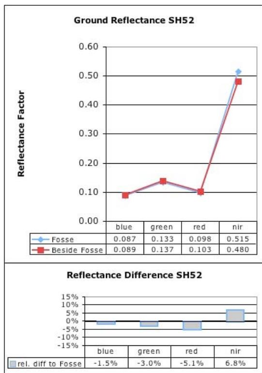
Figure 9. ADS40 SH52 ground reflectances of detected fosses compared to the surroundings
