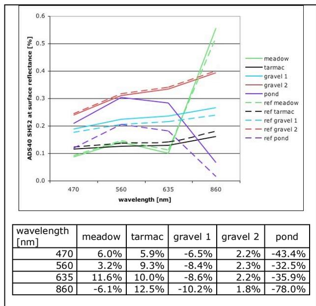
Figure 4. Comparison of ADS40 and ASD-spectrometer at surface reflectance of reference targets, ADS40 sensor head SH52, September 2007, empirical line corrected with ASD targets ,tarmac', ,gravel 1' and ,gravel 2' of September 2007
