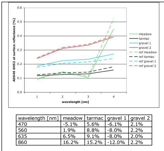
Figure 5. Comparison of ADS40 and ASD-spectrometer at surface reflectance of reference targets, ADS40 sensor head SH40, July 2007, empirical line corrected with ASD targets ‘tarmac’, ‘gravel 1’ and ‘gravel 2’ of September 2007
