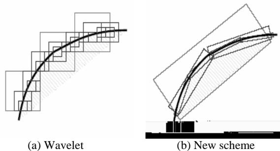
Figure 1. Wavelet versus new scheme: illustrating the successive refinement by the two systems near a smooth contour, which is shown as a thick curve separating two smooth regions?
