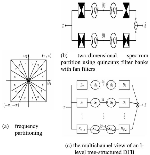
Figure 3. The directional filter bank
