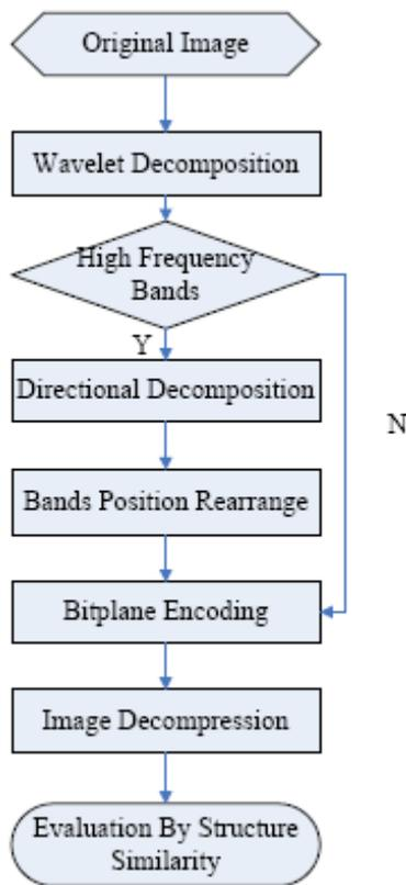
Figure 2. The structure of our compression system
