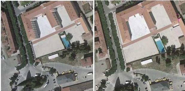
Figure 9.- Example of True Orthorectification using the solution Altas-LRTO.
