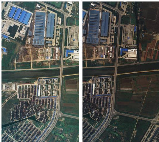
Figure 8. The deviate colour problem in digital aerial image
