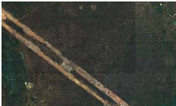
Figure 12. The seamline between mosaic orthophoto
