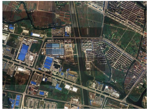
Figure 9. Colour is different between aerial photos, some of them are green, and others are yellow, the result of mosaic orthophoto has blocks
