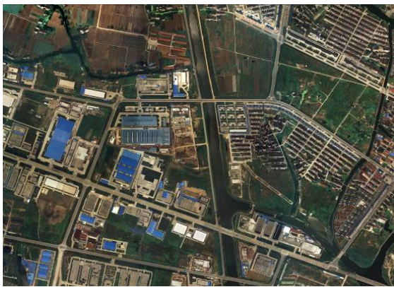
Figure 11. The result after wallis filtering, the blocks in figure 9 is removed after wallis filtering
