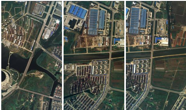
Figure 10. Left is stand image, middle and right is the wallis filtering result of image in figure 8
