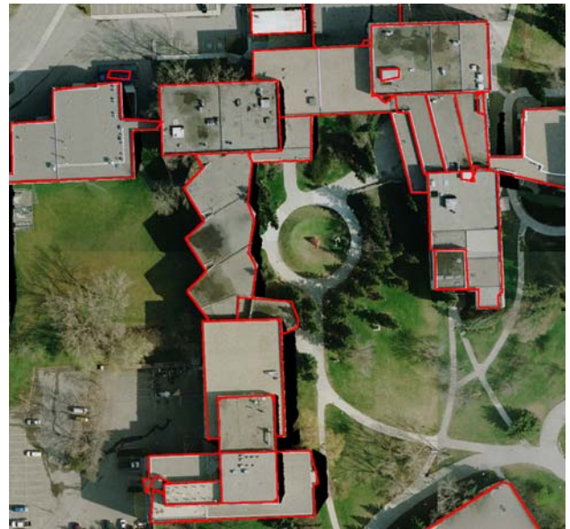
Figure 14. Projected rooftop boundaries onto the orthophoto
