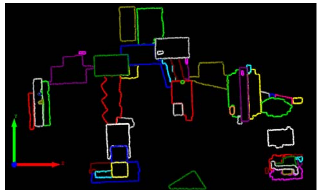
Figure 11. Intermediate boundaries produced by using the modified convex hull algorithm.
