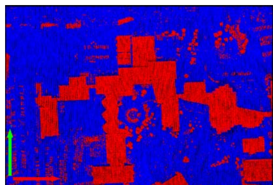
Figure 4. Separated ground and non-ground points.
