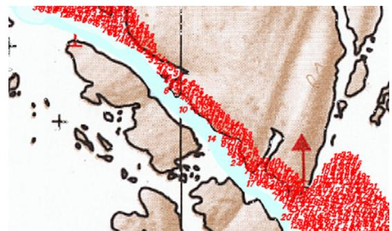
Figure 3: Differences between the old chart no. 1212 and a set of newly measured multibeam data (shown in red). It is evident that the coastline registrations need adjustment.
